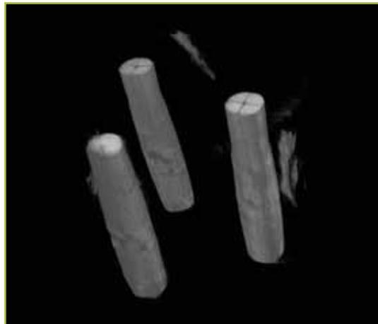
Figure 14. Slice planes applied to the virtual volume display reveal internal features of components such as the gaps in the joints of the conductors.
