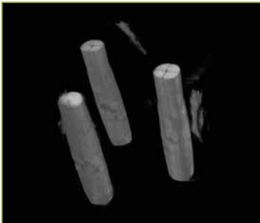
Figure 13. The oil and insulation have been subtracted from the virtual volume display to isolate and highlight the conductors.
