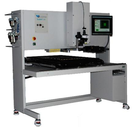
“The Summit LXi has been the leading platform for large board rework for many years,” explains Senior Systems Engineer, Ernie LaFleur. “The system was designed from the ground up for large boards. It has the structural integrity and heating capacity to meet the process requirements for the largest boards we have seen while maintaining the accuracy and reliability our customers expect.”
