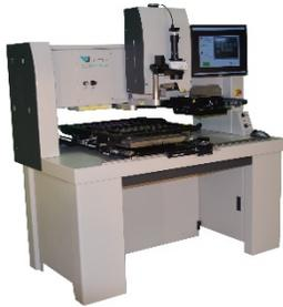
Based on the popular Summit 1800i, the new Summit 2200i offers additional automation. VJE has maintained the benefits of high efficiency convection heating, precision placement and the renowned 1-2-3-Go interface, coupled with a second rework head to allow continuous process from removal, to site dressing and component replacement. Fiducial recognition and automatic alignment eliminate operator intervention and allow multiple components to be reworked consecutively.
